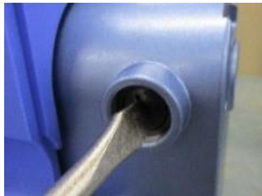
2. Remove the carbon brush mounting screw with a screwdriver.
