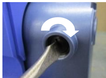
5. Screw in the carbon brush mounting screw. If there is any uncomfortable feeling when screwing in, do not screw it in but remove it again. There is a possibility that the metal part of the carbon brush will be deformed.
