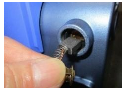
3. Pull out the carbon brush and insert a new carbon brush.
